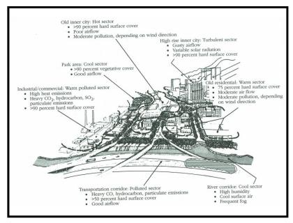
Figure 7. Climatic conditions near the ground in differnt sectors of a city. Conditions vary with surface cover, solar dadiation, airflow, and air pollution, among other things [14]
