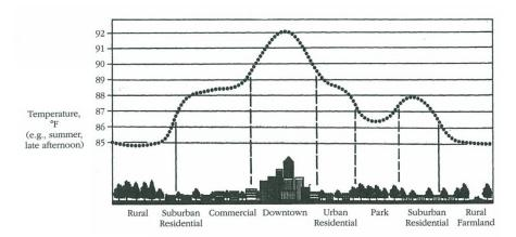
Figure 6. The schematic representation of the temperature profile of the urban heat island and its variation with the type of the elements in the urban area [14].
