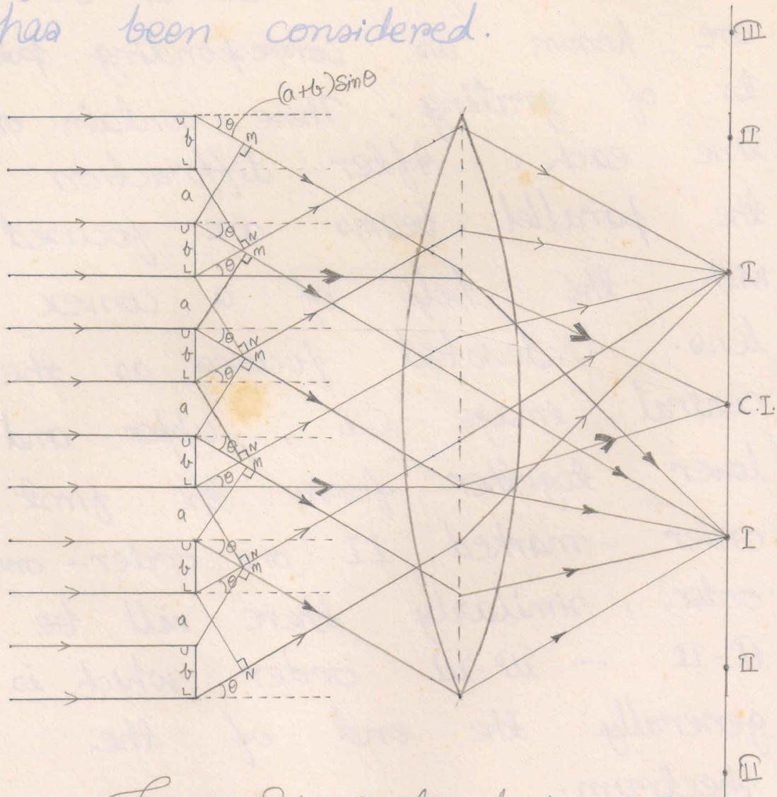
Figure 2: Sectional view of plane grating.
